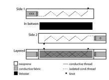
Materials: neoprene, conductive thread, piezoresistive material (velostat, eeonyx nonwoven or eeonyx stretch), conductive fabric (silver stretch), fusible interfacing
